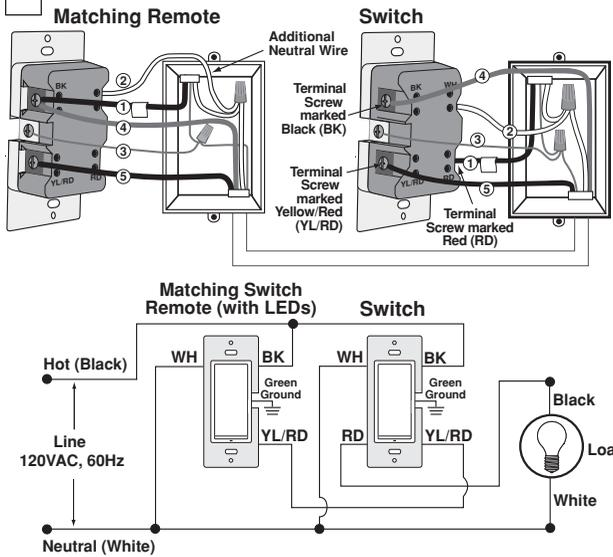
**NOTE:** The switch **must** be installed in a wall box that has a Load connection. The matching remote must be installed in a wall box with a Line Hot connection and a Neutral connection. A Neutral wire to the matching remote needs to be added as shown.
