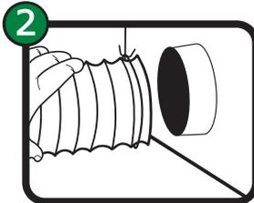
Attach one end of flexible duct to exhaust outlet pipe using clamp (Not Included) and tighten.
