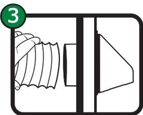
Attach the other end of flexible duct to vent pipe using clamp (Not Included) and tighten.
