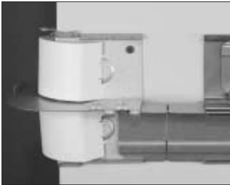
**Step 2.** Leaving Coupling loose, mate DS4000 Base section to installed Fitting. Using up to 4" [102mm] of lateral adjustment provided by Couplings, align Mounting Hole with Wall Stud. Secure to wall using #8 Fasteners 48" [1.2m] apart. Tighten Coupling Screws.
