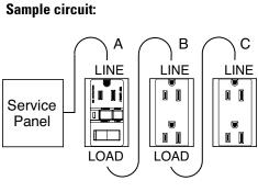
Placing the GFCI in position A will also provide protection to "load side" receptacles B and C. On the other hand, placing the GFCI in position C will not provide protection to receptacles A or B. Remember that receptacles A, B, and C can be in different rooms.
