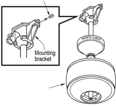
Partially loosen 2 of the set screws on mounting bracket corresponding to the slotted holes on the canopy upper ring. Remove the other 2 set screws. Save screws.
