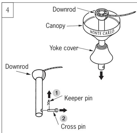
Remove preassembled keeper pin and cross pin from downrod. Place downrod over canopy and yoke cover
