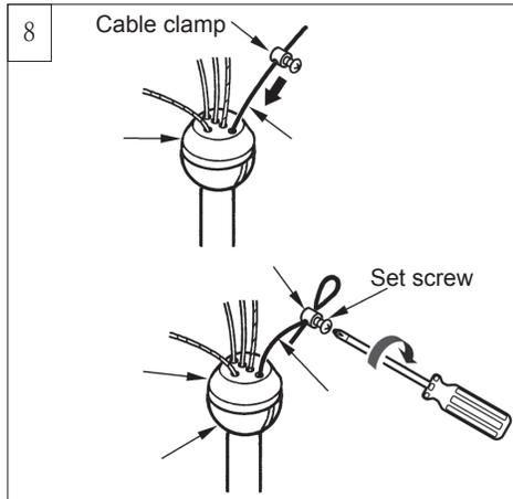
Install cable clamp. Cable clamp provided. Slide cable clamp over the safety cable and feed end of cable into clamp hole and firmly tighten the set screw.
