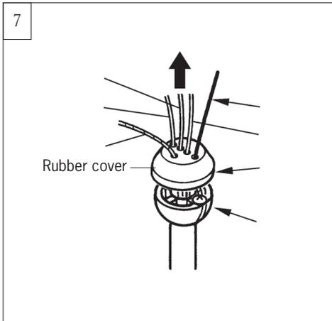
Thread lead wires, grounding wire and safety cable through watertight rubber cover, then place the rubber cover onto hanger ball on downrod. Rubber cover provided.
