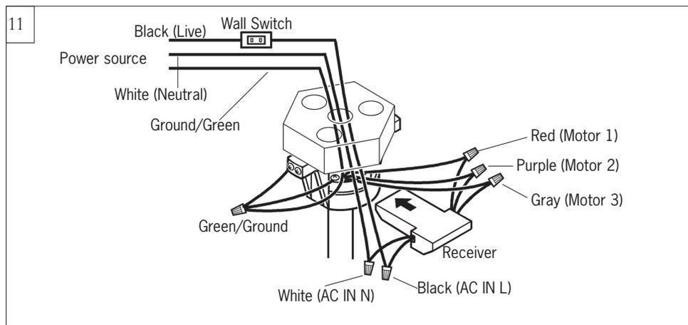
Make wiring connections using wire connectors provided as indicated above.
