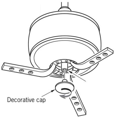
Install a decorative cap onto motor shaft by turning clockwise until tight.
