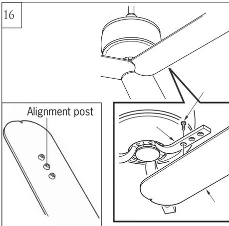
Install blade, aligning 3 alignment posts on blade with the holes in blade bracket, then install it with set screws provided. Repeat this process for remaining blades. Tighten all screws securely.
