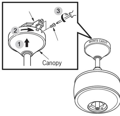
Raise canopy to mounting bracket, aligning loosened screws in mounting bracket with slotted holes in canopy. Twist canopy to lock. Reinstall the screws removed in step 12 and tighten all screws securely.
