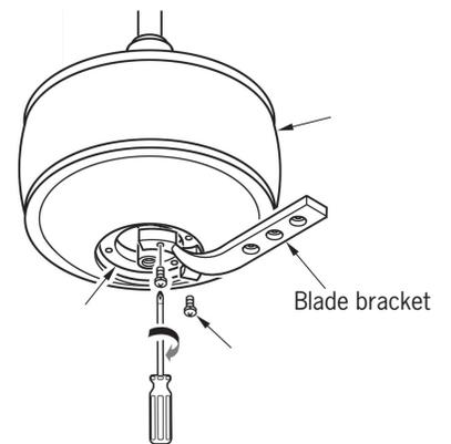
Install blade bracket onto motor with set screws provided. Repeat this process for remaining blade brackets. Tighten all set screws securely.
