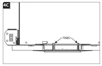
The top portion of the alignment tabs on the plaster ring should be broken off to avoid interference with the light module. Bend the tabs back and forth inside the housing to break the tabs.
