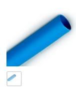
$3M^{\scriptscriptstyle\mathsf{TM}}$  FP-301 Heat Shrink Tubing is a general-purpose, thin-wall tubing that provides a balance of electrical, physical and chemical properties, making it perfect for industrial and military applications. This tubing has a 2:1 shrink ratio and provides flame-retardant insulation for 600V-rated applications. It has a flexible polyolefin construction that offers moisture-seal
