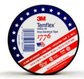
3M™ Temflex™ Vinyl Electrical Tape 1776 is a good quality, economical general-purpose vinyl insulating tape. It has excellent resistance to abrasion, moisture, alkalies, acid, copper, corrosion and varying weather conditions. It is a polyvinyl chloride (PVC) tape that is flame-retardant and conformable. Provides excellent mechanical protection with minimum bulk.
