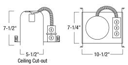
Cut-out: 5-1/2" ID: 5" Housing Length: 10-1/2" Housing Width: 7-1/4" Housing Height: 7-1/2"
