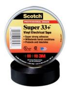
Scotch® Super  $33+^{TM}$  Vinyl Electrical Tape is a premium grade, 7 mil thick, all-weather vinyl-insulating tape. It is designed to perform continuously between a temperature range of 0-220°F (-18-105°C). It has an excellent resistance to abrasion, moisture, alkalies, acids, corrosion and varying weather conditions (including ultraviolet exposure).
