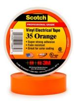
Scotch® Vinyl Electrical Tape 35 is a 7-mil thick polyvinyl chloride (PVC) color-coding tape. It operates over a wide range of temperatures – between 32–220°F (0–105°C). Outstanding electrical and mechanical properties make this tape excellent for use in phase identification, color coding of motor leads and piping systems, and for marking safety areas.
