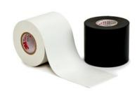
Scotch® Fire-Retardant Electric Arc Proofing Tape 77 is designed to protect most types of electrical cables when exposed to potential failures in an adjacent cable. Its specially formulated adhesive expands in fire to form a thick char buildup between the flame and the cable. The resulting firewall acts as a heat shield and flame barrier, thus protecting the nearby cables and accessories.
