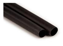
3M<sup>™</sup> ITCSN Heat Shrink Cable Sleeve is a heavy-wall sleeve that provides abrasion, corrosion and chemical resistance. This sleeve has a 3:1 shrink ratio to offer electrical insulation for 1 kV-rated applications. It features a cross-linked polyolefin construction that provides moisture-seal protection.
