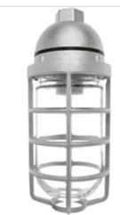
Pendant mount, die cast aluminum construction. Medium base socket, 1/2" or 3/4" NPS pendant thread and a variety of globes. incandescent lamp A21 for 100 Series, PS25 for 200 Series. Lamp not supplied.
