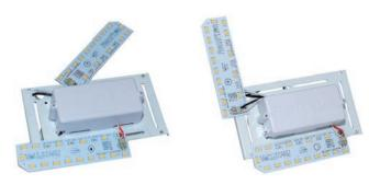
The LEDSR features a patent-pending design which allows the two LED boards to be easily oriented to achieve the desired position to fit a wide variety of shapes and sizes. Simply remove the plastic pin affixing the board in postion and the board can pivot freely. The LED board's mounting screw may be also be removed and reafixed to the slots on any side of the mounting plates for increased flexibility.
