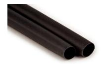
3M<sup>™</sup> ITCSN Heat Shrink Cable Sleeve is a heavy-wall sleeve that provides abrasion, corrosion and chemical resistance. This sleeve has a 3:1 shrink ratio to offer electrical insulation for 1 kV-rated applications. It features a cross-linked polyolefin construction that provides moisture-seal protection.
