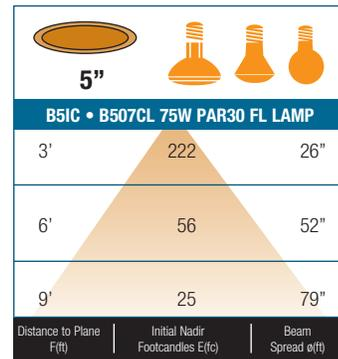
BEAM DIA. MEASURED AT 50% OF NADIR F.C.
