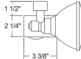
**Line Voltage PAR38****Construction** Polycarbonate body with painted formed steel shade.
