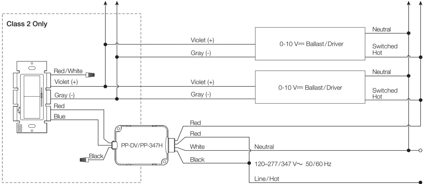
**Dimming With ON/OFF Control For Drivers Which Support Dim To OFF Capability**
