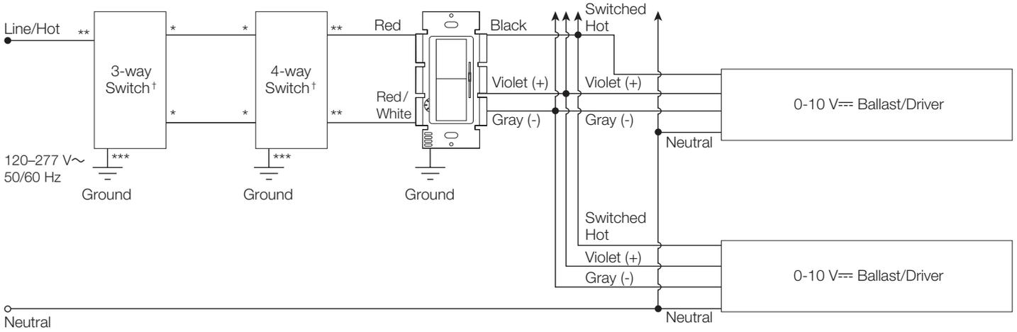
**Note:** For 4-way wiring, control must be installed line side or load side. It cannot be installed in the 4-way location.
