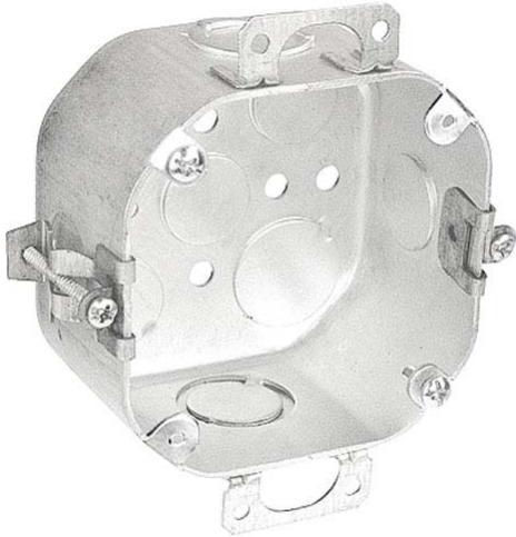
2-1/8" deep, 4" octagon boxes with (2) 1/2" Side Knockouts and (3) 1/2" & (2) 3/4" bottom have dual direction (4) 8-32 threaded mounting tabs with old work clips to add exit signs, scone lights or cameras to existing walls or ceilings. Garvin Industries' deep, octagon boxes are made with a versatile combination head screw. They also come with labor saving installation and mounting tabs that align with most lighting fixtures.
