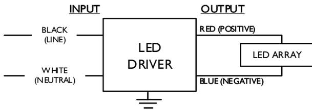
Input and output use lead-wires.
