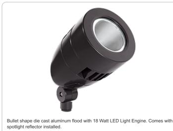
**Driver Info** LED Info Constant Current Watts: 18W Type: 120V: 0.17A Color Temp: 5000K 208V: 0.11A Color Accuracy: 68 CRI 240V: 0.10A 100000 L70 Lifespan: 277V: 0.09A Lumens: 1.997 Input Watts: 20W Efficacy: 101 LPW Efficiency: 91%
