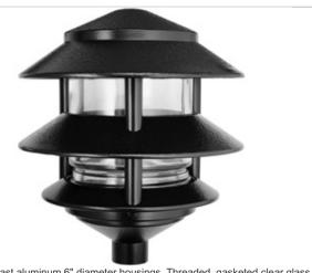
Rugged die cast aluminum 6" diameter housings. Threaded, gasketed clear glass globe for durable weatherproofing and easy relamping. 1" long, 1/2" threaded nipple included for easy mounting. 75 Watt max. Incandescent lamp not supplied. Fluorescent lamp supplied.
