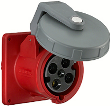
Watertight IEC Pin and Sleeve Receptacle, 3P4W, 60A 3PH 250V
