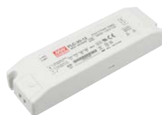
LED-DR30-12 12V DC Class 2 hardwire power supply 100-240V AC input, 1-30 watts 6-1/4"L x 1-1/4" H x 1-3/4"W c/UR/us Recognized for dry locations Can be used with AL-PWM-6A dimmer which consumes 3 watts
