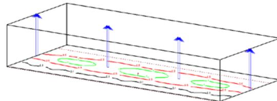
For ceiling mounted applications, simply aim the lamp heads straight down to create a uniform well-lit path of egress.
