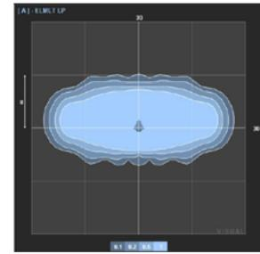
The ELMLT features a linear distribution which maximizes uniformity and fixture-to-fixture spacings.
