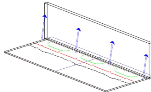
For wall mounted applications, a slight tilt away from the wall creates a uniform well-lit path of egress. Traditional circular pattern optics require multiple iterations using complex angles to meet the NFPA 101 requirements of 1fc-average, 1fc-minimum, and 40:1 maximum-to-minimum uniformity.
