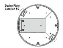
NOTE: Standard size for device plates for Plate Location 4 is 5 7/32" [132mm] x 2 3/4" [62mm].
