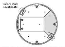
NOTE: Standard size for device plates for Plate Location 3 is 5 7/32" [132mm] x 2 3/4" [62mm].
