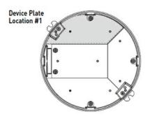
NOTE: Standard size for device plates for Plate Location 1 is 6 11/32" [161mm] x 2 3/4" [62mm].
