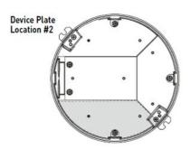
NOTE: Standard size for device plates for Plate Location 2 is 5 7/32" [132mm] x 2 3/4" [62mm].
