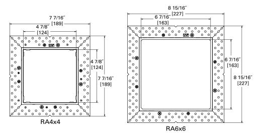
ORDERING INFORMATION EXAMPLE: PN6S1H42E + E6SL2GMWRL + RA6X6 = 6" square, non IC, air tight housing platform, UNV 120/277V electronic ballast for (1) 26W DTT or 26/32/42WTTT lamp, diffuse glass lens shallow optical element, matte white finish, rimless adapter for 6" elements.
