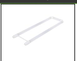
The ETi 15 watt 1800 lumen LED T8 U Bent tube offers exceptional performance for precision lighting applications. These 6" Leg Spaced LED tubes are high quality replacements for fluorescent lamps and are available in 4000K. They are UL Classified for use in damp locations and are RoHS complaint with no lead or mercury. Non-dimmable. Warranty period 5 years or 60 months. Suitable for installations from –13°F to 113°F.
