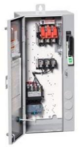
Non-reversing motor starter Size 0 Three phase full voltage Solidstate overload relay OLRelay amp range 3-12A 110-120/220-240VAC 60HZ coil Combination type 30Amp fusible disconnect 30 Amp /600V fuse clip Enclosure NEMA type 4/12 Water/dust tight weather proof Standard width enclosure
