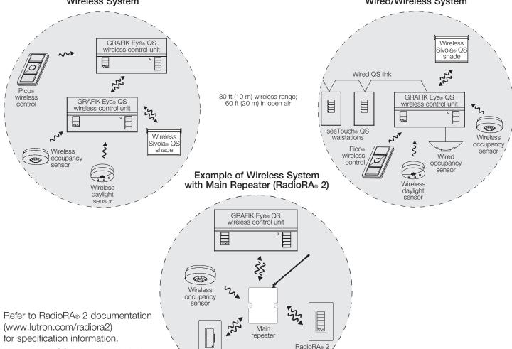
Note: Wired QS link is disabled when the GRAFIK Eye® QS control unit is added to a RadioRA® 2 system.
