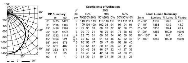
2AVL4 50L MDR LP835, 5095 delivered lumens, test no. 69071P9, tested in accordance to IESNA-LM79.
