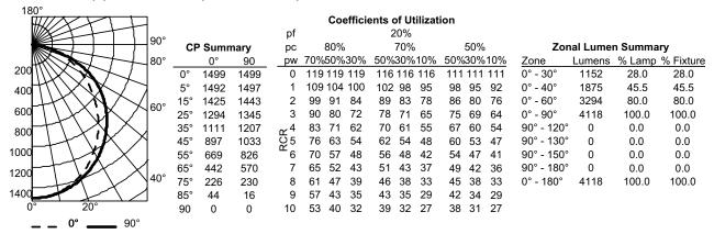
**2RTL4 48L LP835**, 4,786 delivered lumens, test no. LTL25588P8, tested in accordance to IESNA LM-79.
