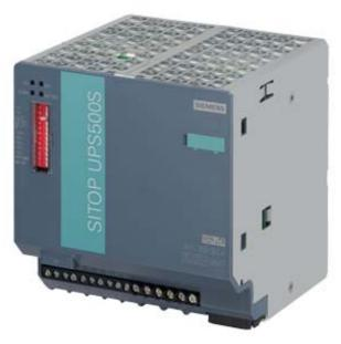
SITOP UPS500S BASIC UNIT 2.5 KWS SITOP UPS500S service-free uninterruptible power supply with USB-interface basic unit 2.5 kWs input: 24 V DC output: 24 V/15 A DC degree of protection IP20
