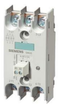
Semiconductor relay, 3-phase 3RF2 30 A / 40  $^{\circ}$ C 48-600 V / 4-30 V DC 3-phase controlled Ring cable connection Blocking voltage 1200 V
