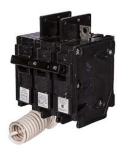
Siemens Low Voltage Molded Case Circuit Breakers General Purpose MCCBs - Type BQ, 2-Pole, 120/240VAC are Circuit Protection Molded Case Circuit Breakers. 2-Pole Common-Trip circuit breaker type BQ. Rated 120/240V (100A) (AIR 10 kA). Special features: Load side lugs are included.
