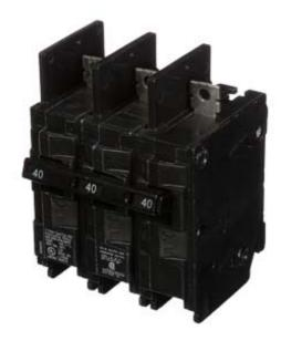
Siemens Low Voltage Molded Case Circuit Breakers General Purpose MCCBs are Circuit Protection Molded Case Circuit Breakers. 3-Pole Common-Trip circuit breaker type BQ. Rated 240V (040A) (AIR 10 kA). Special features: Load side lugs are included.
