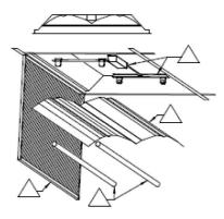
**Kit includes:** (1) reflector, (1) MV-N Ballast, (2) aluminum brackets, (2, 4 or 6) lamp holders, (4) Tek screws (1) Disconnect
