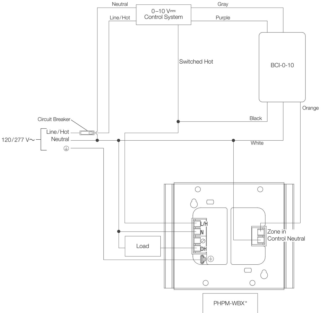
\* When the BCI-0-10 is being fed with 120 V~ from the 0-10 VDC control system, use the PHPM-WBX-DV-WH. When the BCI-0-10 is being fed with 277 V~ from the 0-10 VDC control system, use the PHPM-WBX-277/DV.
