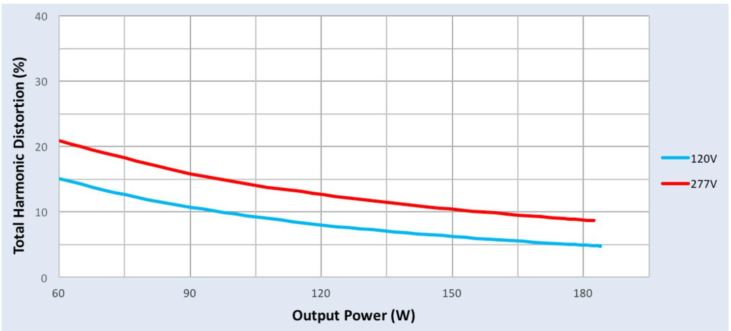
\* Power Factor and Total Harmonic Distortion graphs are shown for combined output power of both channels.
