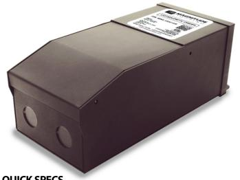
Magnitude's M300L24DC is the most compact LED driver on the market with a magnetic transformer core. It is equipped with two push-to-reset circuit breakers on the input and output, which protect both the load and driver. The driver is encased in a coated metal box that includes 4 knock-outs on the bottom to enable easy installation that complies with electrical code requirements.
