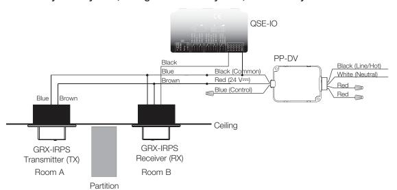
Note: Diagram represents a single partition. A QSE-IO will accommodate up to five GRX-IRPS partition sensors (five partitions). A single PP-DV will power one GRX-IRPS partition sensor.
