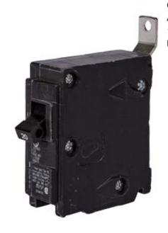
Siemens Low Voltage Molded Case Circuit Breakers Panelboard Mounting 240V Circuit Breakers - Type BL, 1-Pole, 120VAC are Circuit Protection Molded Case Circuit Breakers. Type: HBL Application: Electrical Distribution Standard: UL 489 Voltage Rating: 120V Amperage Rating: 20A Trip Range: Thermal Magnetic Interrupt Rating: 65 AIC Number Of Poles: 1P
