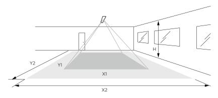
Note: Longer dimension of detection area (Y1, Y2) is parallel to longer dimension of EasySense.
