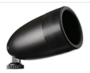
Premium PAR38 Flood with large, molded high temperature black silicone gasket that totally seals lamp. Die cast aluminum housing. EZ Locknut. Suitable for mounting within 4' of the ground. PAR38 or PAR20, 150 Watt max. Lamp not supplied.
