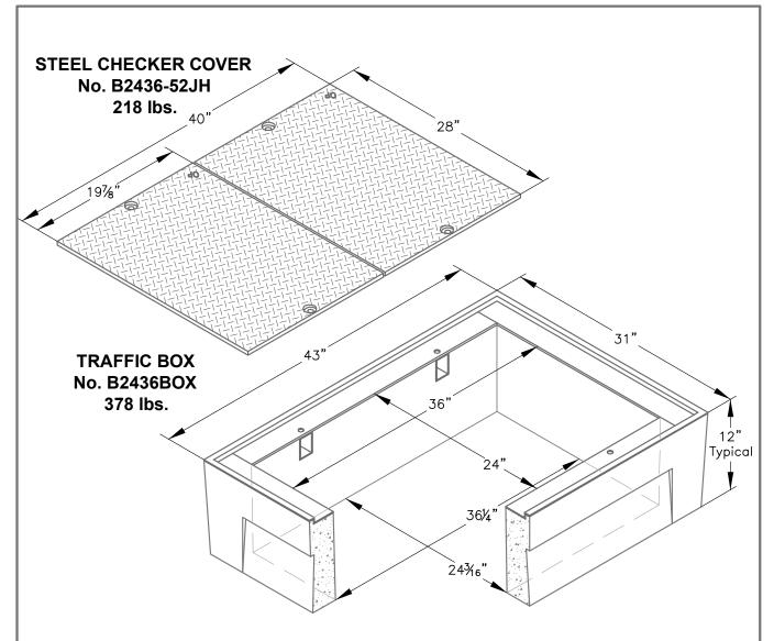
A high density reinforced concrete box with non-settling shoulders positioned to maintain grade and facilitate back filling. Approximate dimensions and weight shown.
