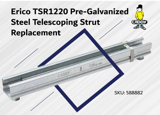
Erico Telescoping strut replacement in pre-galvanized finish, has steel construction for high strength and durability. The captive threaded nuts help in fastening it to threaded rod supports. It can be adjusted to the desired length from 14 to 21.5-inches.
