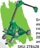
Greenlee Ultra Tugger® Motorized cable puller assembly with mobile versi boom, has polyester composite construction for durability. It offers a pulling speed of 16 FPM at no load, 14 FPM at 2000 lbs, 12 FPM at 4000 lbs, 7 FPM at 6000 lbs and 6 FPM at 8000 lbs.
